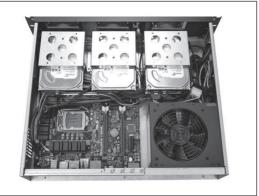
8. For the HDD Cage on the right side, it can take up to 2x 3.5" HDD or 1x 3.5" HDD + 1x 2.5" HDD. You can place the Cage vertically when you are using a standard ATX PS2 power supply (140x150x86 mm).
