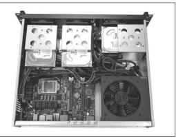
You can also place the HDD Cage horizontally if you use a longer ATX power supply (165x150x86 mm).
